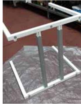
2. Place and tighten the screws inside the aluminum bars (4pcs M6x25).
